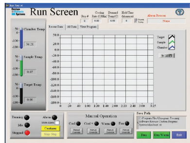
Run screen provides all details of actual freeze runs during operation, plus all manual override controls.
